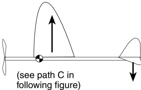
This airplane is properly balanced. The lift of the wing tries to rotate it nose down and the lift of the horizontal stabilizer tries to rotate it nose up. The moments created by the two forces are in balance and the airplane glides properly.
