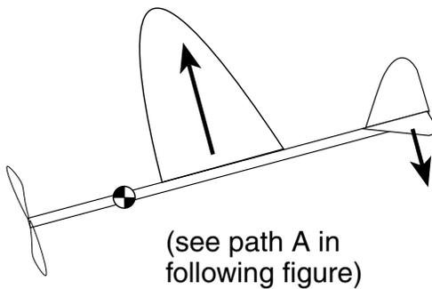
The wing on this airplane is too far back. Because the moment arm is longer, the lift of the wing causes the nose to drop more than the horizontal stabilizer lift can raise it, just like the heavier student on the teeter-totter.
