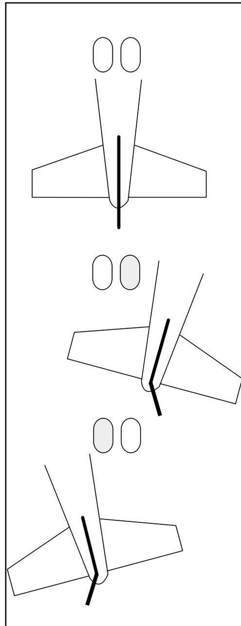
**Aileron:** A control surface attached to the wing causing it to roll left or right.
