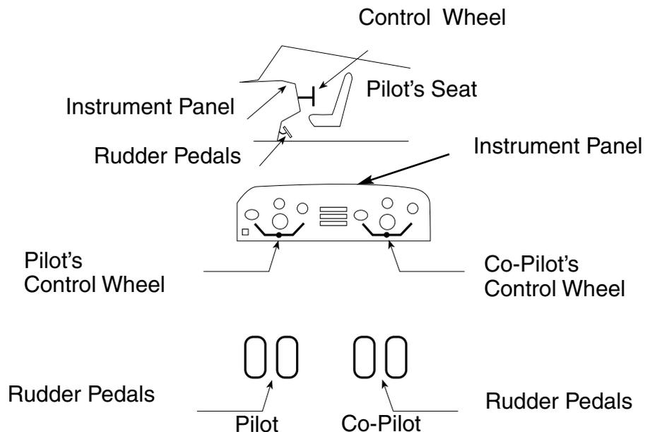
plane to do what it does. That is accomplished through the flight controls. Inside the cockpit, the pilot has a set of flight controls that move the ailerons, elevator and rudder.
