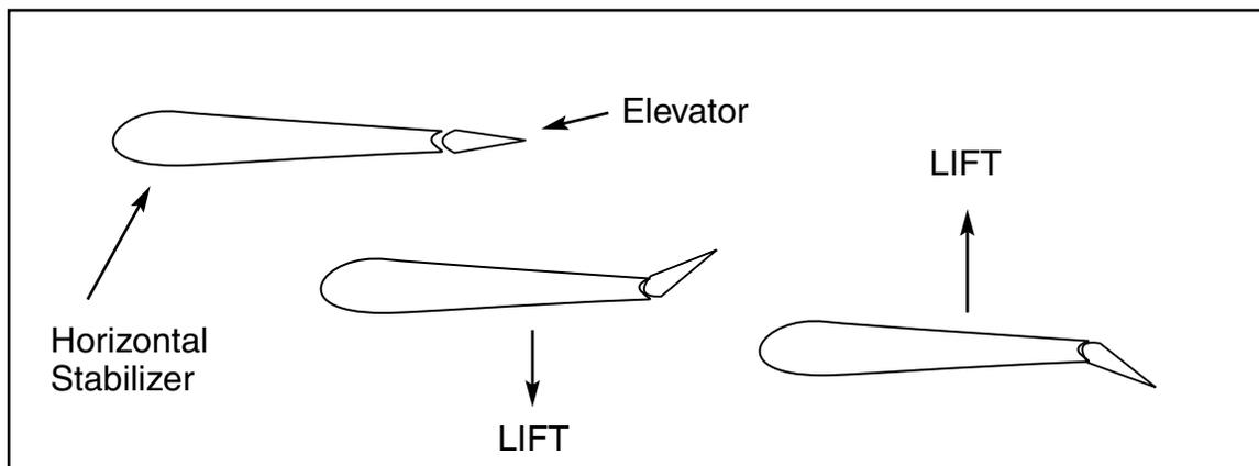
**Rudder:** The rudder is connected to the vertical stabilizer and is controlled by the pilot to move left and right. The vertical stabilizer along with the rudder form another small wing. As the rudder moves left or right, it changes the lift produced and causes the nose of the airplane to swing (yaw) left or right. The diagram for the elevator is identical to the rudder, except it would be viewed from above instead of the side.
