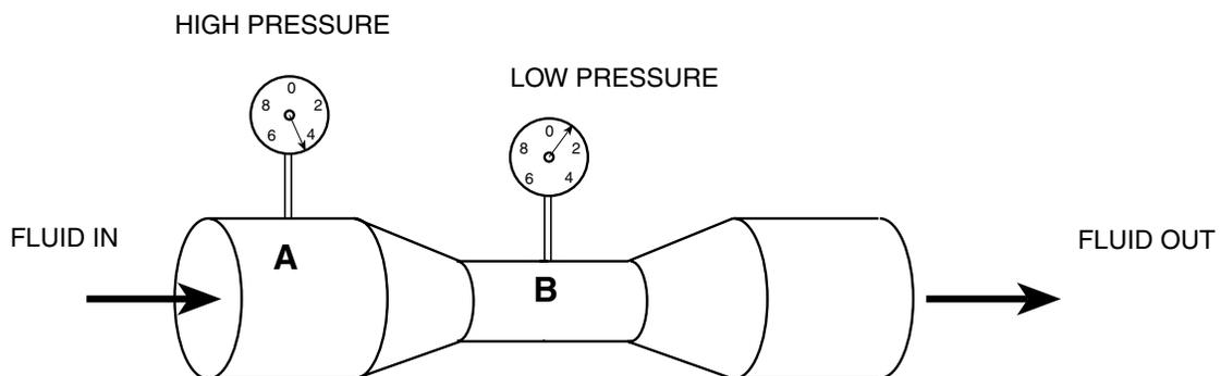
A wing produces lift using the same principle. Instead of a pipe, we use an airfoil. An airfoil is the cross sectional shape of a wing if you cut through it. A typical airfoil is shown on the next page. The upper camber of the airfoil changes the flow pattern of the air across it, like the garden hose nozzle changes the flow pattern of the water
