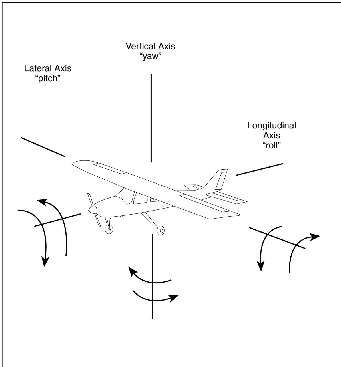
Motion about the lateral axis (pitch) is caused by movement of the elevator. When the elevator moves down, the stabilizer and elevator form an airfoil that produces lift causing the tail to rise. The airplane pivots about the center of gravity and causes the nose to go down. The airplane is now in a dive. When the elevator deflects up, the opposite occurs, forcing the nose up and the airplane is now in a climb.
