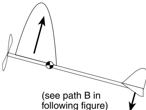
Now the wing is too far forward and causes the nose to rotate up. The tail lift also causes the nose to rotate up.
